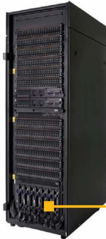
IBM PureData System for Analytics uses Field Programmable Gate Arrays (or FPGAs) that are programmed to handle large volumes of data very efficiently. These FPGAs eliminate all unnecessary I/O calls, and then further reduce and filter the data as fast as it streams off the disk. This removes I/O bottlenecks and frees up downstream components such as the CPU, memory and network from processing unnecessary data, creating a significant turbocharger effect of system performance.
